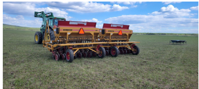
Figure 2: HAYBUSTER No-Till drill used for seeding of the legume mixture
